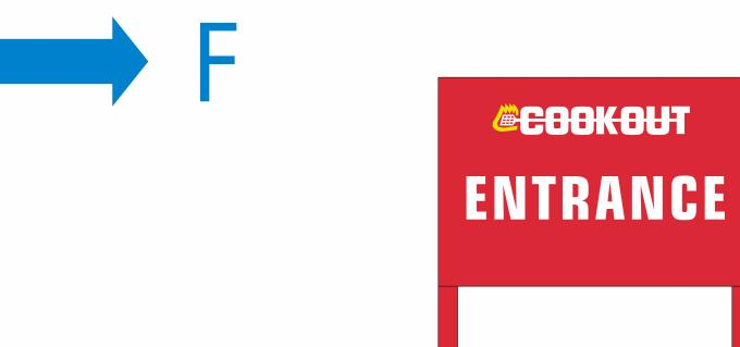
(2) 3' x 2' (3' high when installed) powder coated aluminum drive-way entrance signs
