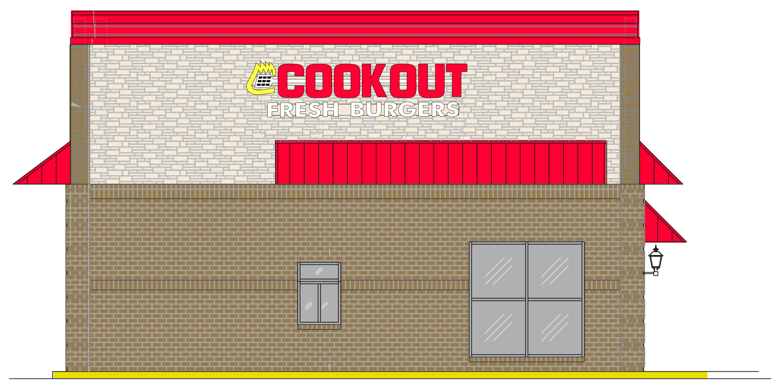
Front of building 15' 2'6" COOKOUT 14" FRESH BURGERS 14' - UL listed, LED lighted channel letters - Powder coated aluminum race-way mounted scale 1/2" = 1'
