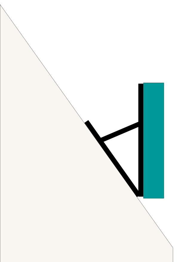
powder coated steel angle bracket to compensate for the roof's pitch
